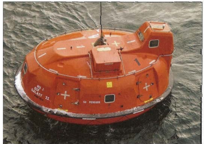
A Whittaker single davit lifeboat (TEMPSE). This is one type of lifeboat used when it becomes necessary to evacuate an offshore platform. Photo courtesy of the Bercha Group.
