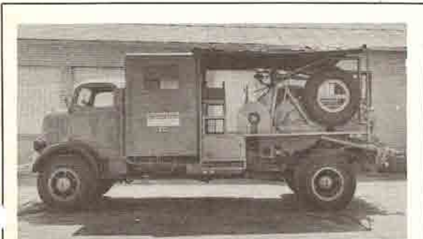
Schlumberger Unit No. 273, just off the assembly line, similar to the first Schlumberger units in Canada, with the roll-down canvas sides and un-insulated metal recording shack.
