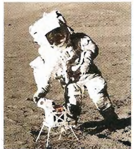
Figure 3. Harrison "Jack" Schmidt deploying the Surface Electrical Properties equipment (SEP) during Apollo 17 mission, 1972.
