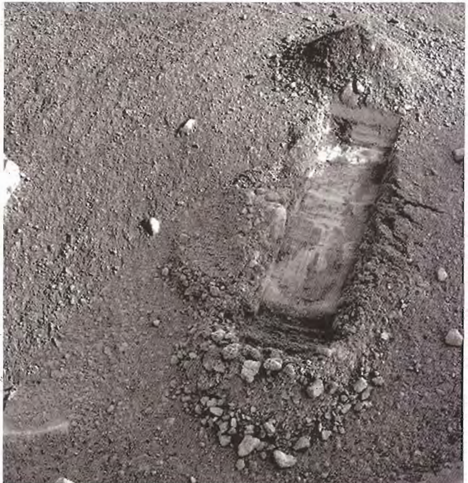
Figure 11. True colour photo image of a Mars Phoenix trench. White areas are believed to be water ice, as they appear to sublimate slowly after exposure to the Martian atmosphere. Samples were processed in the Thermal Evolved Gas Analyzer (TEGA).
