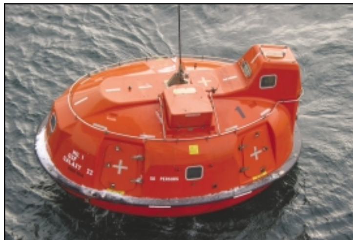
A Whittaker single davit lifeboat (TEMPSE). This is one type of lifeboat used when it becomes necessary to evacuate an offshore platform. Photo courtesy of the Bercha Group.
